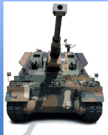
KRAB – 155 mm self-propelled howitzer Maximum speed, road – 60 km/h Fire zone – 40,000 m Max. rate of fire – 6 shots/min for 3 min Additional machine gun – 12.7 mm WKM-B Manufacturer: HSW S.A., Cooperation: ZM Tarnów S.A.
