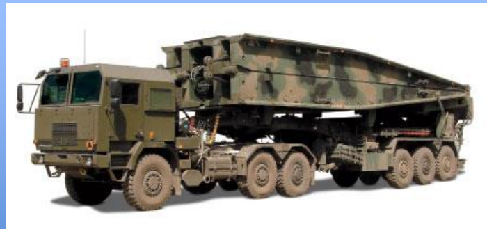
MS-20 DAGLEZJA – accompanying bridge on wheeled chassis
