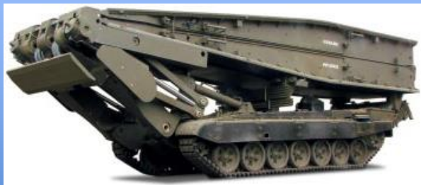
MG-20 DAGLEZJA-G – assault bridge on tracked chassis
