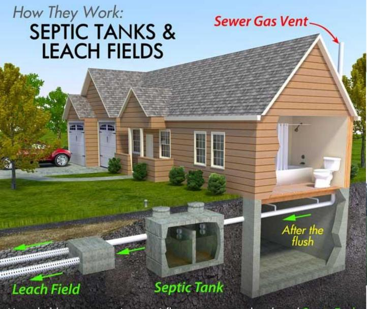
Household wastewater (sewage) flows into a two-chambered Septic Tank. In there, solid waste falls and collects at the bottom for later pump-outs. The wastewater then continues to a Leach Field of perforated pipes for natural absorption into the soil.
