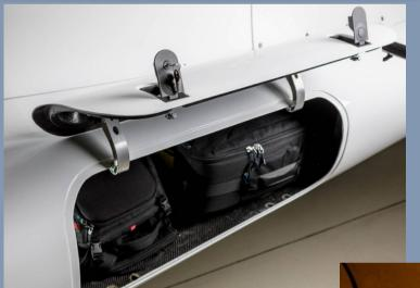
Safe door-closing system-11 pins, ensuring airtightness.
